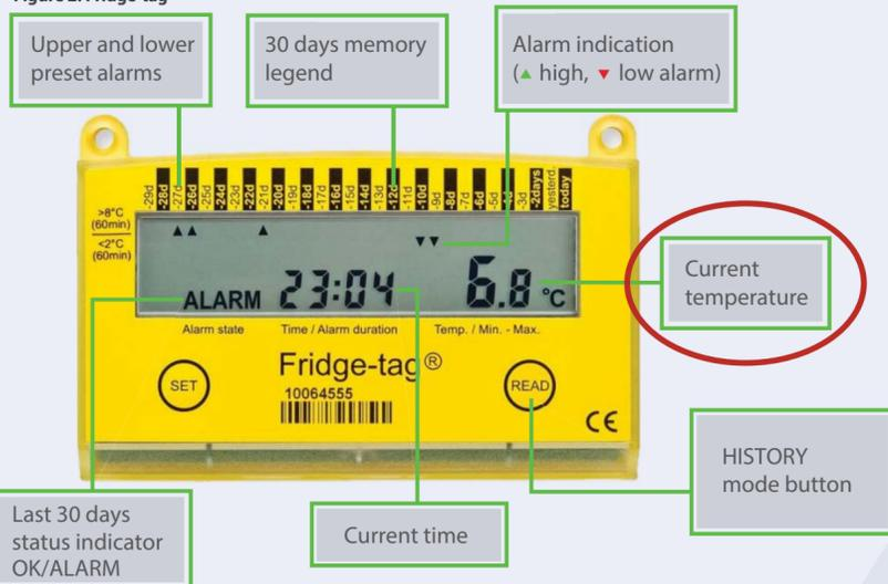
Figure 3. Fridge Tag Temperature Recording Sheet
